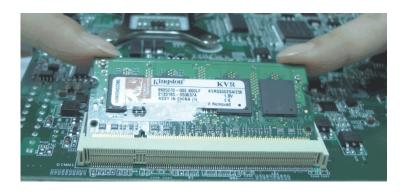
6. Push down the module until the clips at each end of the socket lock into position. You will hear a distinctive "click", indicating the module is correctly locked into position.
